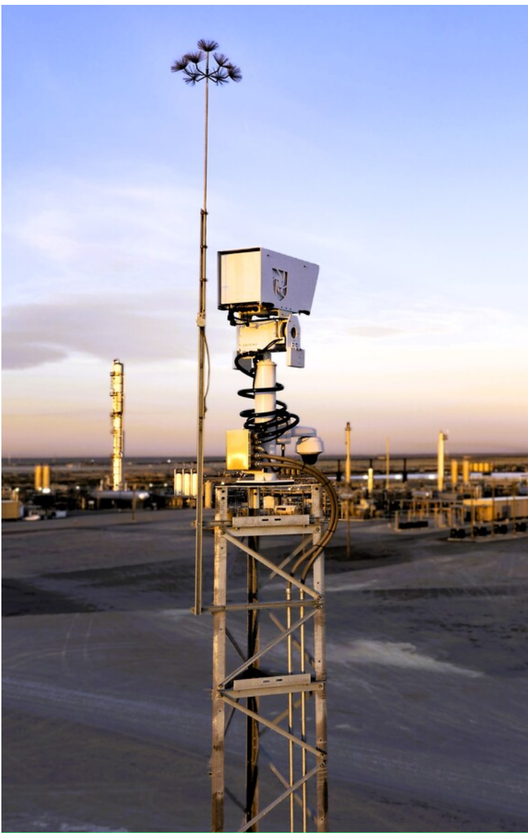
Rebellion Gas Cloud Imaging Camera, Pecos Bend Plant
